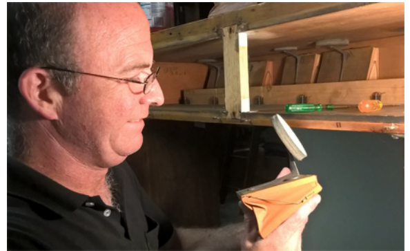
Todd Milnar examining the spring and pouch for a Sub Bourdon 32
